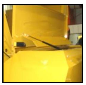
LID NOTE: Make sure the lid opening is facing backward to prevent it from opening while transporting the GT40 Tank/Trailer.
