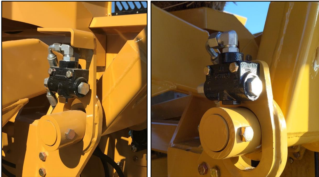
Clamps lift up in slot, activating the valve. Lowering the forks resets this.
