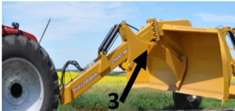
Figure 1.2.1: Shows the safety locks marked by arrows
